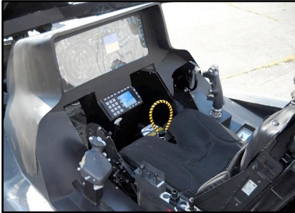
The refinement of techniques developed in the VAAC Harrier fed into the F-35B, making the control systems simple to use, and rendering the cockpit conspicuously simple compared to the Harrier.
