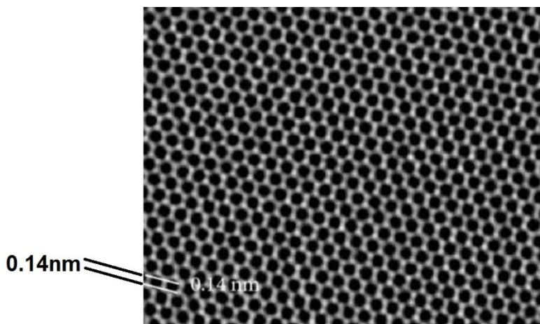
The lattice-like structure of graphene is comparable to a natural honeycomb.
