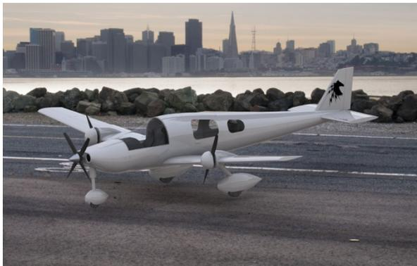
The HEGAAsus family of aircraft brings the latest development in hybrid powertrain technology to the 4 and 6 seat general aviation market, carrying its passengers up to 1000nmi at speeds in excess of 200kts. Thanks to its hybrid powertrain, which optimises energy utilisation through two electric motors and a diesel engine, fuel burn is reduced by up to 50% compared to its nearest competitors. The HEGAAsus is due to enter into service in 2028 and aims to mark a step change in air travel.
