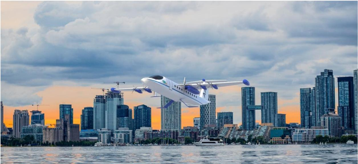
The AAT (Amphibious Air Taxi) Platypus is a new amphibious aircraft which will replace existing aircraft with such capabilities as well as unlock new commuting opportunities in and around urban areas. The aircraft has a passenger capacity of 32 and maximum useful range of 500km however its primary mission is that of making frequent short hops.
