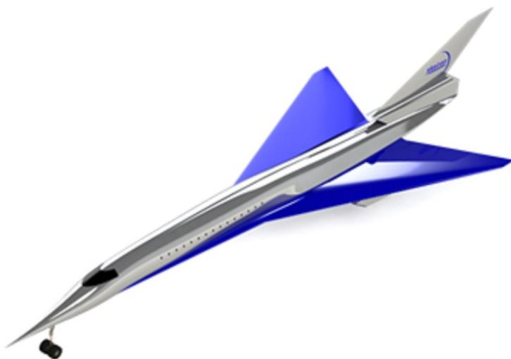
list was considerable: included innovations were a variable-cycle engine, a cruising speed of Mach 2.5 cruise, and the specification of a synthetic vision system (that alleviated the need for a droop nose). Commercial attributes were outlined too, and operations were planned around a 6hr operation that would allow an out and back cycle daily: an objective that would ensure utilisation was adequate to meet the seat-cost targets.
