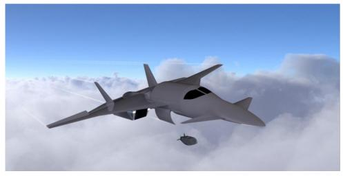
Argo is a collaborative project between Loughborough University and Virginia Tech to develop a supersonic platform with both military and civilian applications. Differing by only the cabin or payload module, Argo can deliver 25 passengers or 5000kg of payload at transpacific ranges in just under 100
