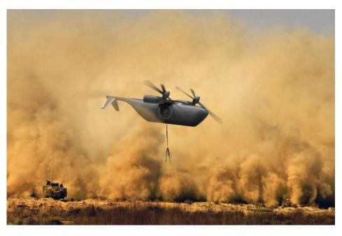
Vanguard Aviation present the FF-12 Griffin, an autonomous tiltrotor cargo aircraft designed and engineered to handle the unexpected. The bespoke tiltrotor powertrain blends the versatility of a helicopter with the efficiency of a fixed wing aircraft. With a military focus the folding wing mechanism enables efficient storage in confined spaces such as aircraft carriers, while its innovative payload handling system
