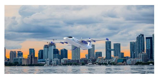
The AAT (Amphibious Air Taxi) Platypus is a new amphibious aircraft which will replace existing aircraft with such capabilities as well as unlock new commuting opportunities in and around urban areas. The aircraft has a passenger capacity of 32 and maximum useful range of 500km however its primary mission is that of making frequent short hops.
